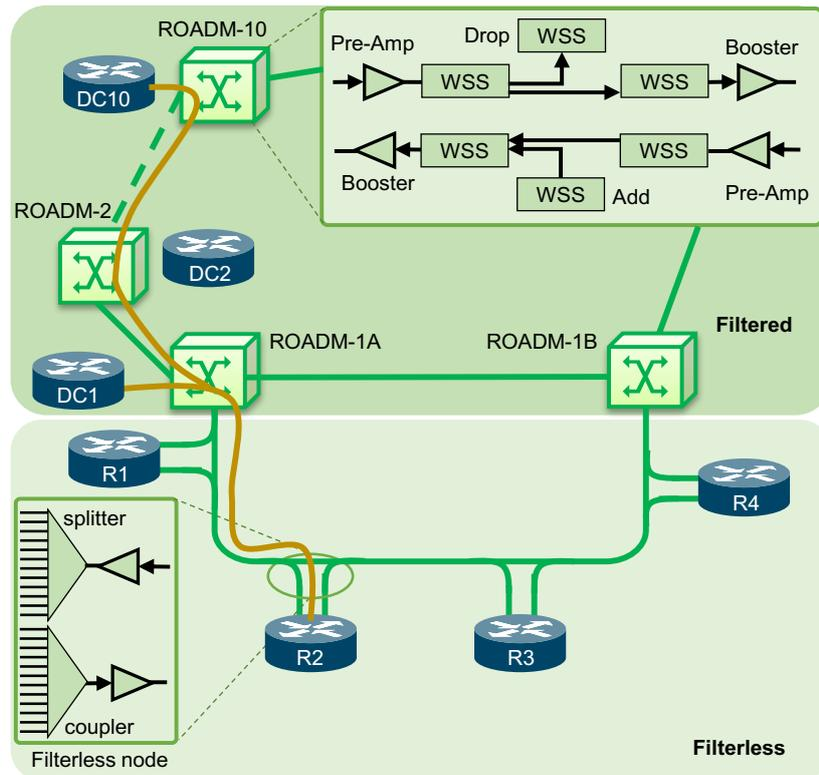
**Fig. 1. Hybrid filterless and filtered-based metro network.**
