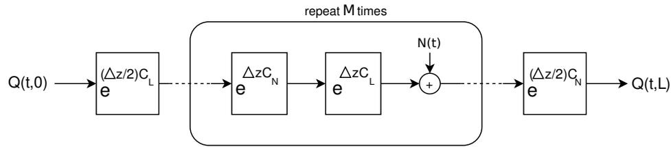
**Fig. 2.** Split-step Fourier method
